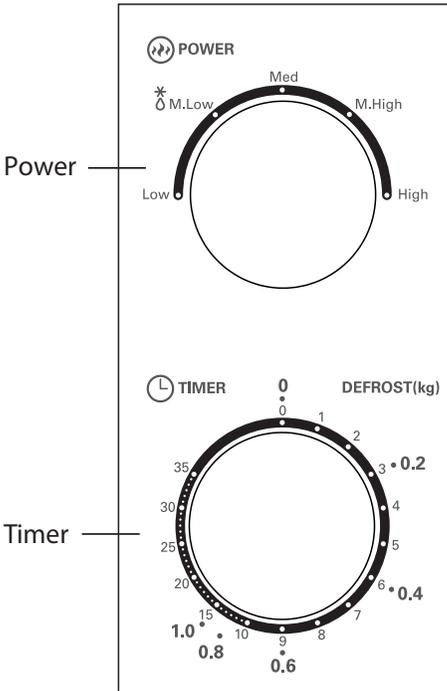
1. To set the cooking power by turning the power knob to the desired level.
