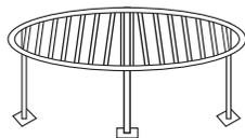
Grill Rack( Only be used in grill function and be placed on the glass tray )
